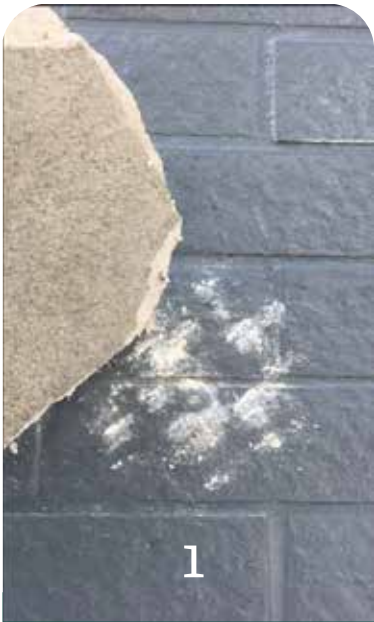
Stone Impact on Diamond Master Snoflex Coating.
